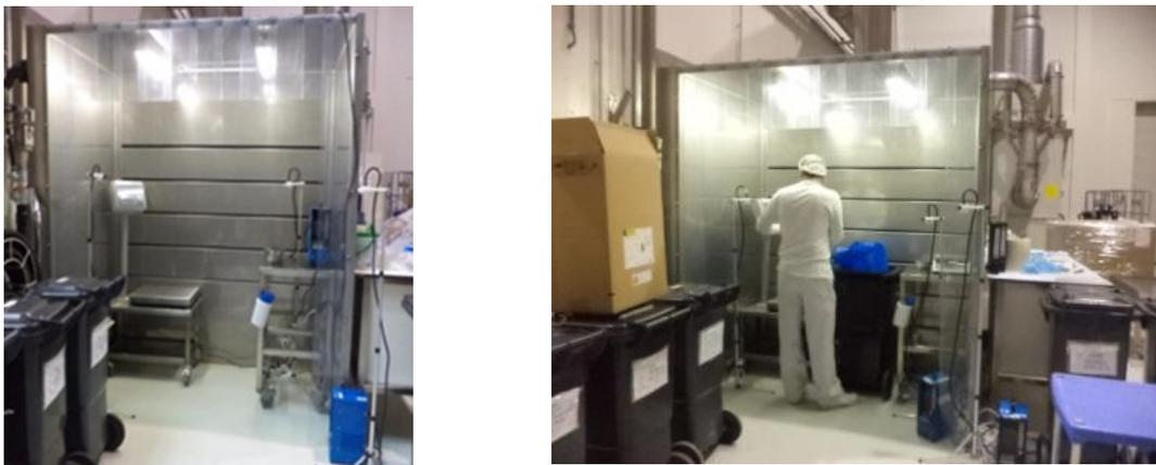
Figure 5. Examples of (pre-) weighing units for enzymes.
