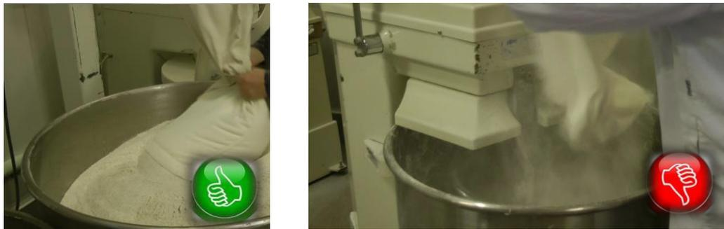
Figure 19. Unloading flour and improvers in mixing bowls: dos and don'ts.
