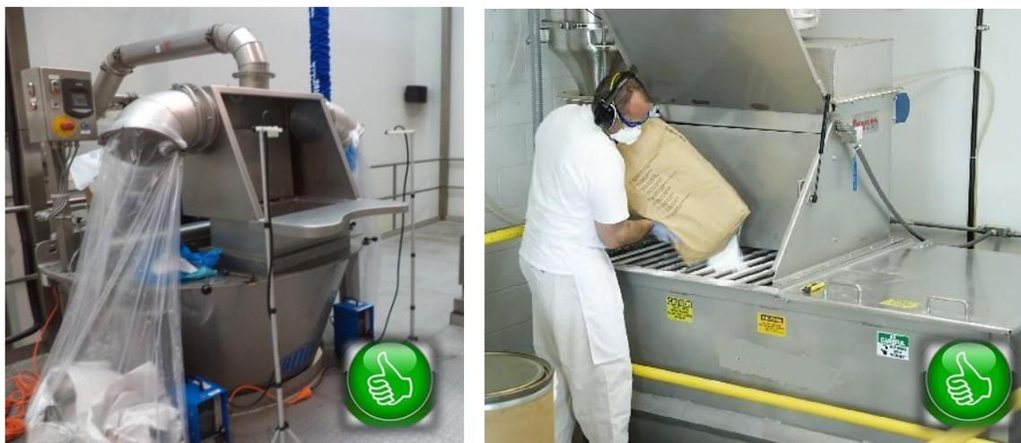
Figure 7. Examples of dumping stations.
