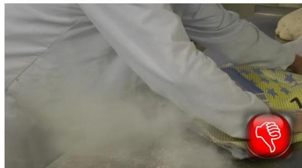
**Figure 21. Safe vs. unsafe removal of empty paper bags from the baking environment.**
