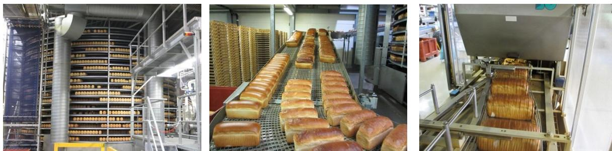
**Figure 16. Conveying final product in industrial bakeries.**
