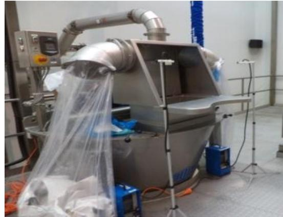
Figure 9. Ventilation principles for paper bag emptying operation (preferably through the back of the unit).
