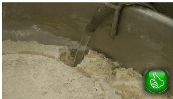
Figure 22. Safe addition of water into mixing bowls without creating dust.
