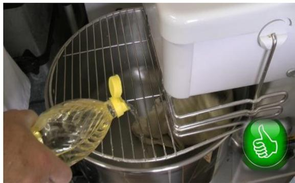
Figure 24. Safe vs. unsafe release of the dough from the mixing bowl.
