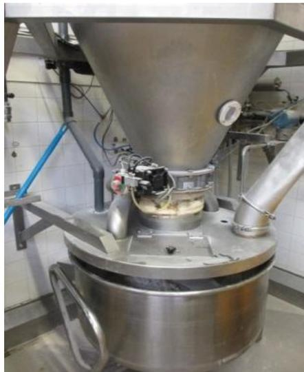
Figure 14. Connection system for silos.
