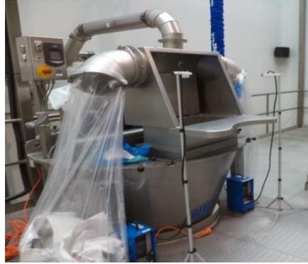
**Figure 2. Automatic disposal unit for empty (used) product bags in a PE-liner.**
